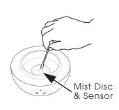
Use a cotton swab to gently clean the Mist Disc and Sensor located at the inside bottom of the base.
