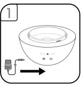
Plug the power to the unit first then connect to wall outlet.
